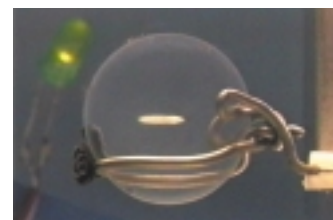
HIFU in action. (Above) Schlieren optical image of the acoustic field shows how the ultrasound energy is focused into a narrow region. (Below) Formation of a HIFU lesion (area of necrotic tissue) within a bovine lens. The treated area is the size of a rice grain.
