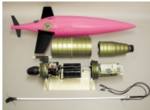
Seaglider components. (From top to bottom: external hull, internal pressure case, internal electronics and mechanics, and antenna.)
