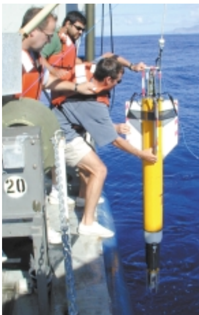
A DAMP recovery. The thin blue line is a loose tether that transmits data and allows the profiler to be cycled continuously behind the ship.
